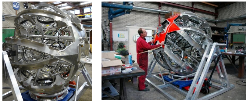
Figure 15 Launching vehicle in rotator (left). Loading the launching vehicle with optical modules on a string structure in the lab (right).
